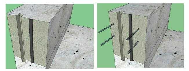
Insure the waterbar is properly placed in the centre of the wall according to instruction and secured into position with at least 75mm of cover.
